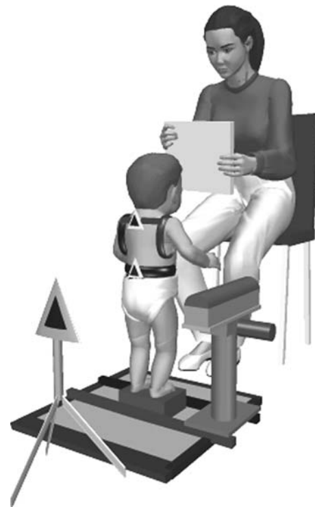
Fig. 1 An infant stands independently on a pedestal in the no-touch condition. An experimenter sits in front of the infant to keep his/her attention in the task. In the touch condition, the infant's hand lightly touches the bar, which is pictured here to the infant's right
